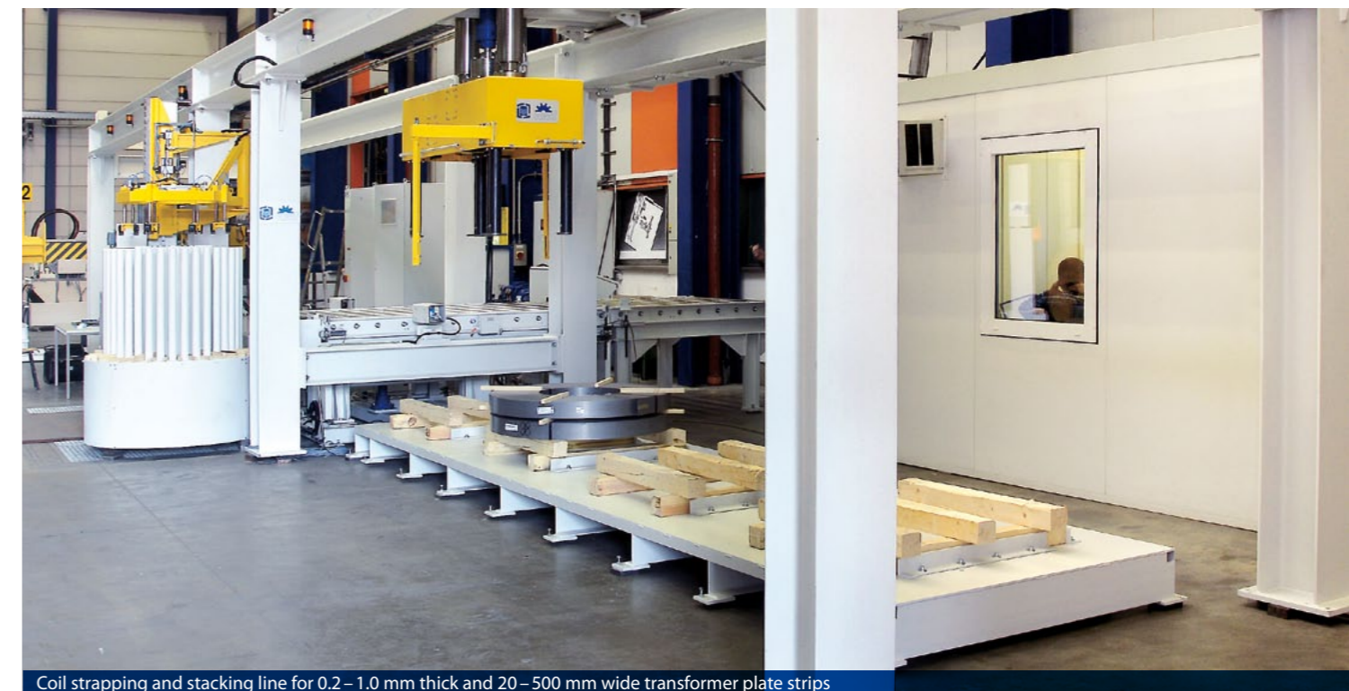
Coil strapping and stacking line for 0.2 – 1.0 mm thick and 20 – 500 mm wide transformer plate strips
