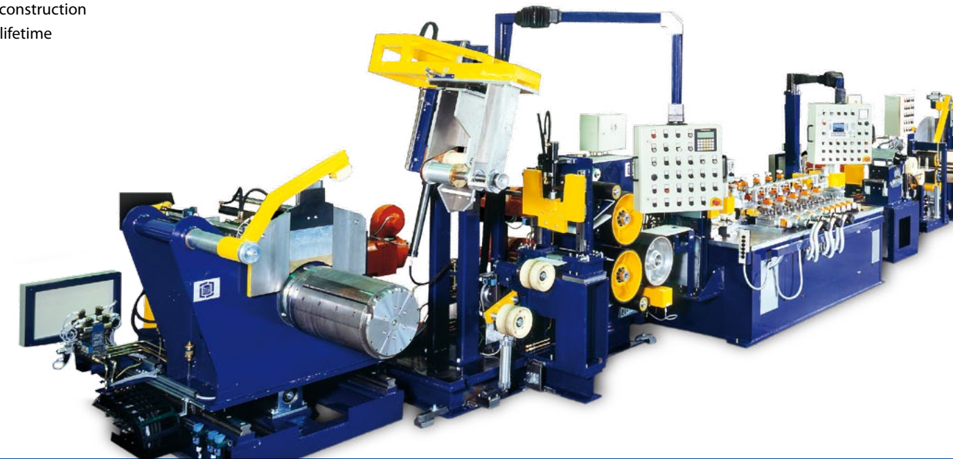
Strip edge trimming line with manual and motor-driven tool adjustment system
